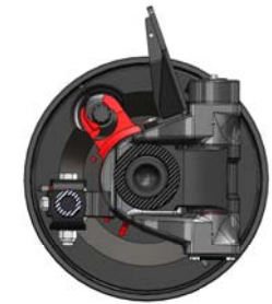
AXLE SHOWN HAS HYDRAULIC RAM ON TOP SO THE AXLE IS FOR UNDERSLUNG SUSPENSIONS
