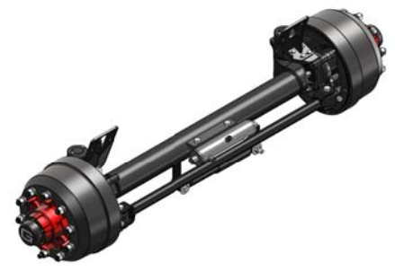
AXLE SHOWN HAS HYDRAULIC RAM ON TOP SO THE AXLE IS FOR UNDERSLUNG SUSPENSIONS
