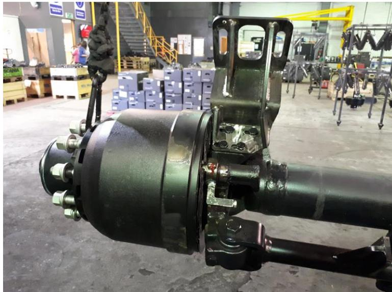
**Stepped ACB design for AIR/HYD chambers on 300 series steer axles**
