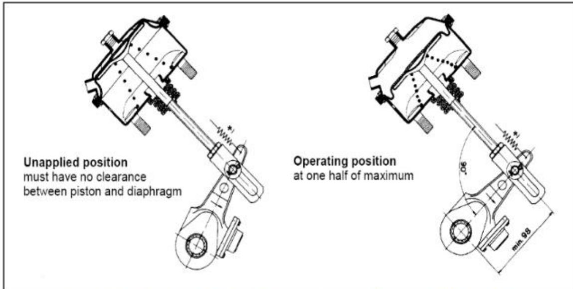
**Slack adjuster and push rod at 90° when brake chamber at half stroke.**
