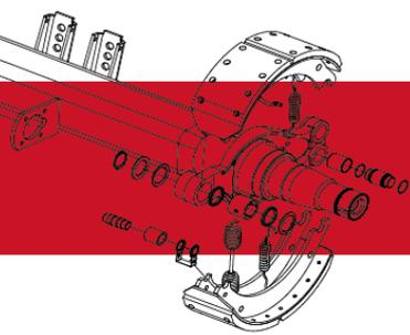
correct length. If the length of the push rod is too long or too short then the braking power can be reduced.
