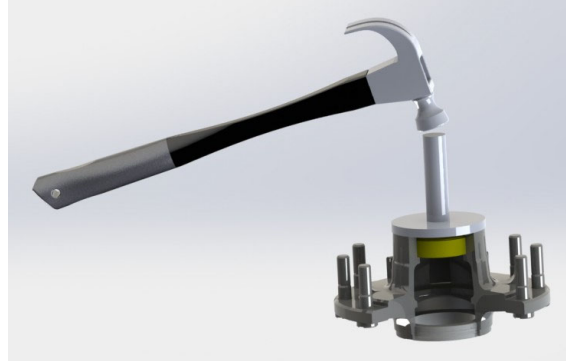
Outer bearing cone being fitted
