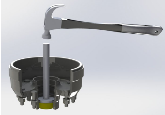
Outer bearing cone being removed.
