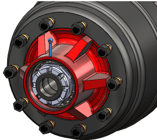
Straighten cotter pin tab's & remove it
