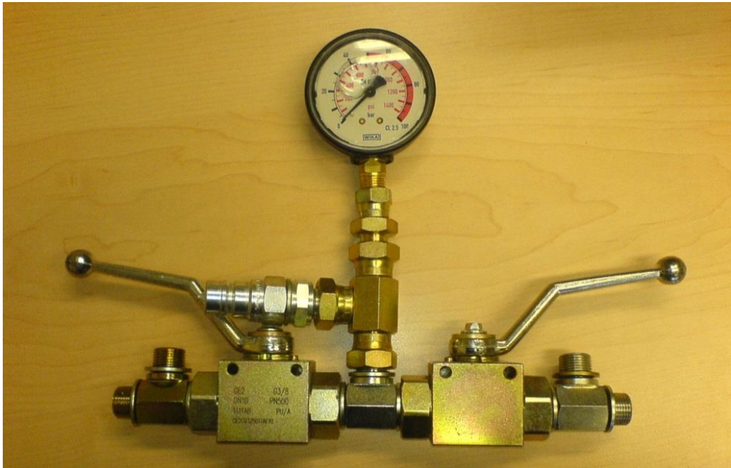
Figure 7 Connecting point for the hand pump + Shut-off valves
