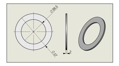
61056 - Camshaft Grease Seal
