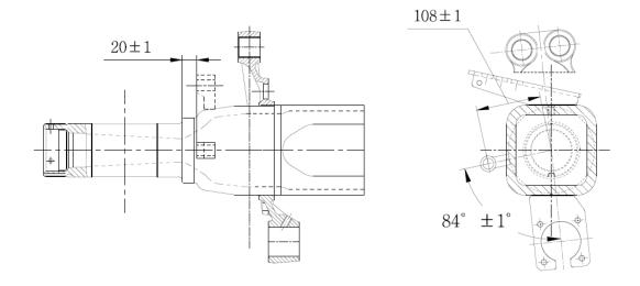
ABS sensor at 216mm PCD Face of sensor block 20mm from large bearing shoulder ABS Block welded 84Degrees from the camshaft axle center line. After fitting ABS sensor check the sensor is working properly.
