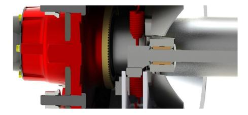
The direction of the grease seals in the anchor bracket is important as well as the position of the beveled washer between the anchor bracket and camshaft head.
