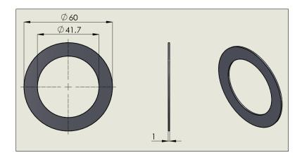
20040 - Camshaft Grease Seal
